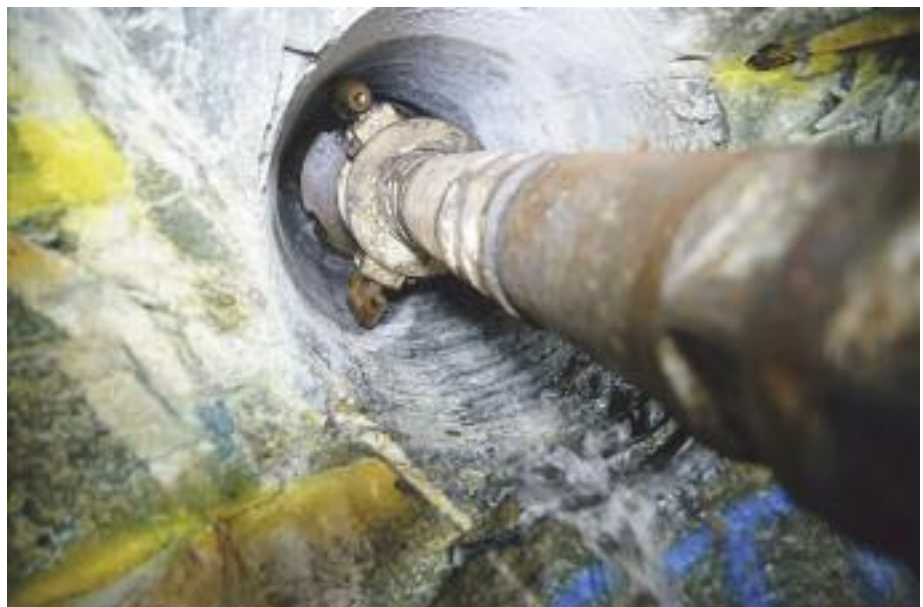
Looking down an AngloGold Ashanti reef boring hole
