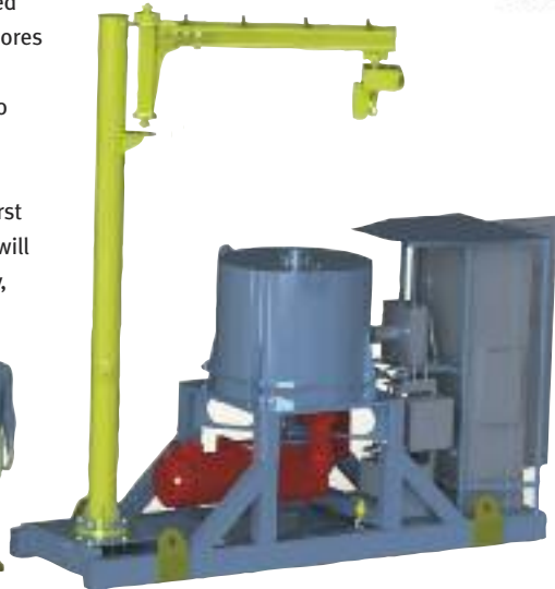
eHPCC: an image representing the machine constructed and scheduled to be commissioned early July 2016 and how eHPCC might be used in a large throughput application. For a small throughput only one feeder and eHPCC might be needed
